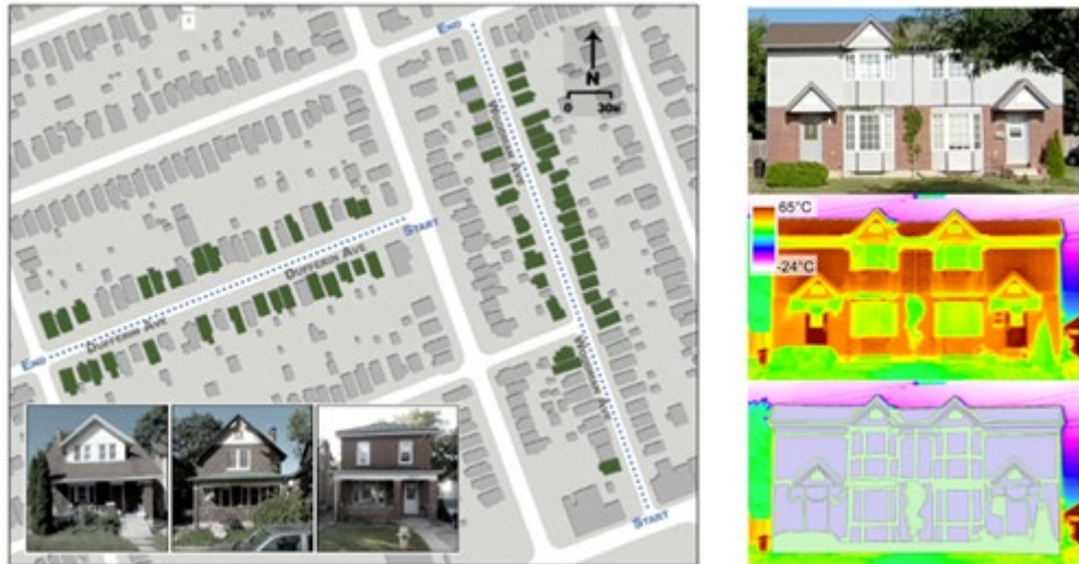
- Figure 7. Map of the mobile traverses (left) carried out in (Hilland & Voogt, 2020) and example of the visible image (top), thermal image (middle), and classified image (bottom) obtained for a west-facing house.
